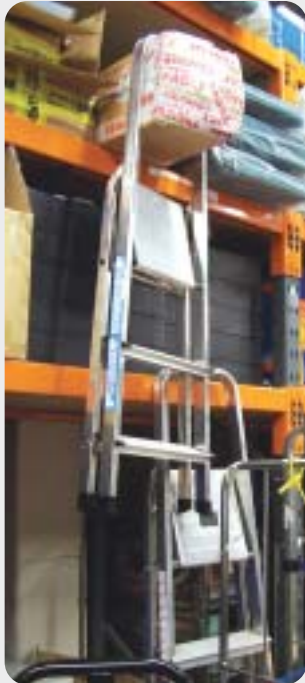
Dangerous situation discovered during an inspection – a stepladder used to access racking.
